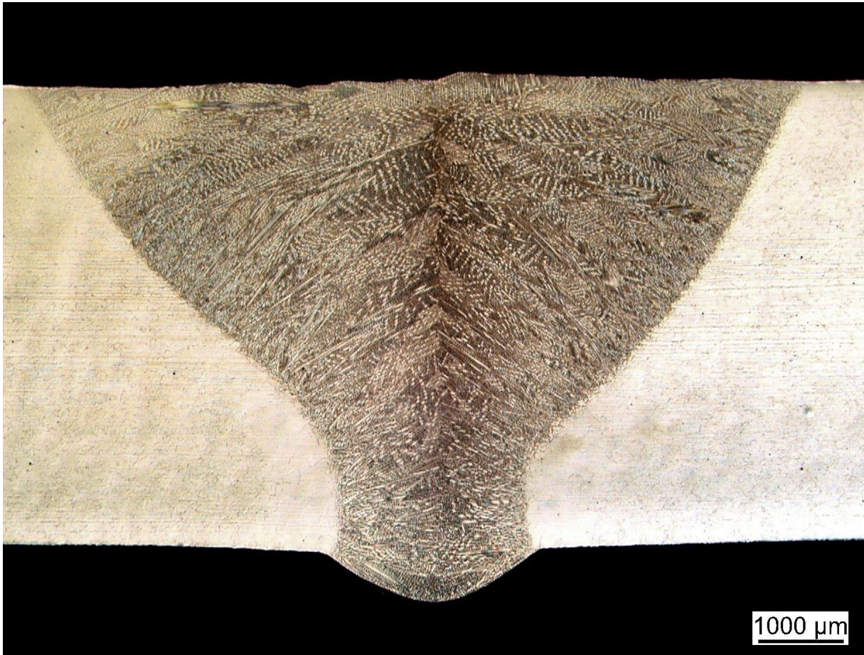
Figure 4: Transversal metallography view of weld seam
